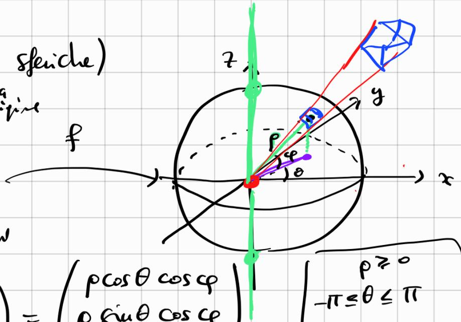
$$\begin{pmatrix} x \\ y \\ z \end{pmatrix} = f(p, \theta, \varphi) = \begin{pmatrix} p \cos \theta \cos \varphi \\ p \sin \theta \cos \varphi \\ p \sin \varphi \end{pmatrix}$$
