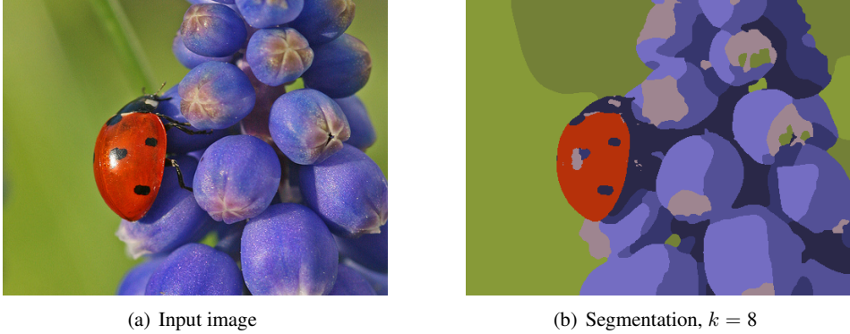
Figure 16. Piecewise constant Mumford-Shah segmentation of a natural image. (a) shows the input image and (b) is the minimizer of energy (4.30). The mean color values c_i of the partitions have been initialized using k-means clustering.
