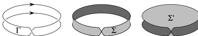
Fig. 6. The surface with minimal area spanning the (oriented) curve \Gamma is the Möbius strip \Sigma . However, \Sigma is not orientable, and cannot be viewed as a current. The mass-minimizing current with boundary \Gamma is \Sigma' .
